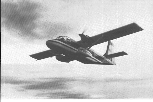
Nomad 22, a twin turbo-prop utility aircraft manufactured at the Government Aircraft Factories at Fishermens Bend. This aircraft, designed to operate economically on short range low density traffic systems, has capacity for twelve passengers, or alternatively 9 cubic metres freight volume.
